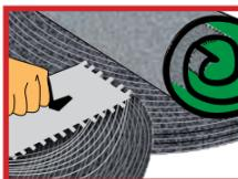
Step 1 - Having trimmed your Prograss, position pieces face up, as they will be installed. Mark a line on the base where a seam will appear, turn back the carpet, spread adhesive over an area about 600mm to 1000mm wide on either side of this line.
