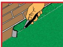
Step 3. – Trim off excess around perimeter. Should you require a neat finish around edges or across doorways, special plastic or metal strips are available from carpet stores.
