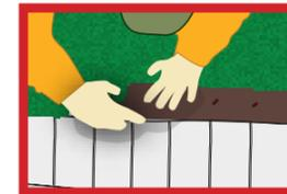
Step 2 - Having trimmed your Prograss (see Trimming & Joining) to approx. 100mm oversize, roll out into position and trim to size and shape.
