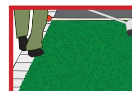
Step 5 - Groom carefully into pile using a stiff bristle broom and making sure it falls to the base of the grass initially and that no pile is tucked under. Continue in layers to within 10mm to 20mm from the top, ensuring that the infill is evenly distributed, using the stiff bristled broom to remove creases or wrinkles as you go. Recheck the edges, trimming the Prograss as necessary and adjusting to have the Prograss level with edging.
