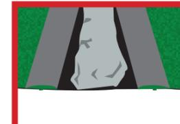
Step 3 - To join, butt two pieces of Prograss together, fold back both pieces and lay joining tape. Use a notched trowel to spread adhesive onto joining tape. Carefully fold both pieces of Prograss together and press into adhesive, making sure no pile is tucked under.
