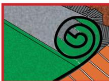
Step 2. – Lay one side of carpet on the adhesive up to the line, then lay the other side up to the line and butt the trimmed edges. Roll back the Prograss that has not been glued down and spread adhesive over the remaining surface, rolling the Prograss down as you go until all carpet has been adhered. Press the carpet firmly into the adhesive and work out any air bubbles with hand pressure or the back of a push broom or roller.
